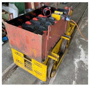
Now completely reassembled, the loco can be easily charged by just plugging in to a 240v supply with a commando connector as seen above.
