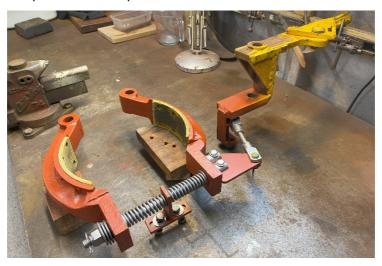
Upon consulting the Operator's Manual 'Brakes' section it could be seen that to correctly adjust the brakes an adjustment stop screw was to be used, this was found to be
