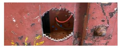
Once all the drilling and fitting out was done and a trial fitment was successfully completed all the batteries, charger, hold down clamps and connecter were removed and the inside of the box was painted with an acid proof bituminous paint.
