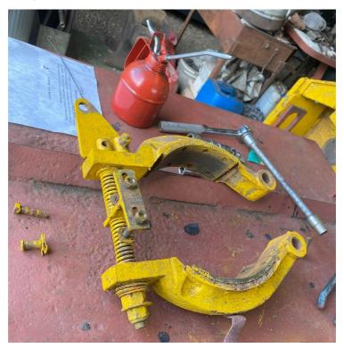
I took the whole assembly home to my workshop and proceeded to fully disable it. When inspected it was clear that it had not been working properly as one of the brake shoes was un-worn and had not been contacting the drum at all!
